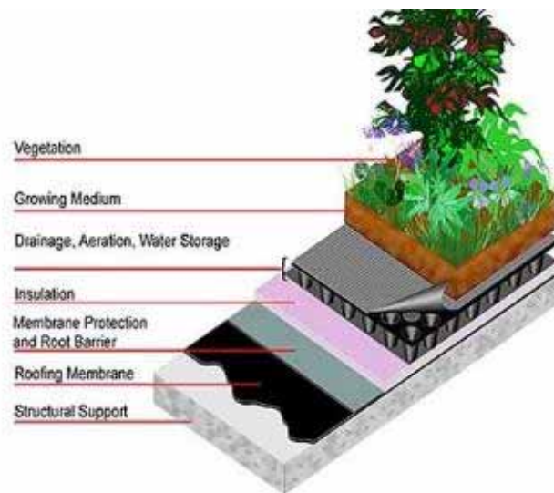
Figure 8. The various layers forming the green roof
