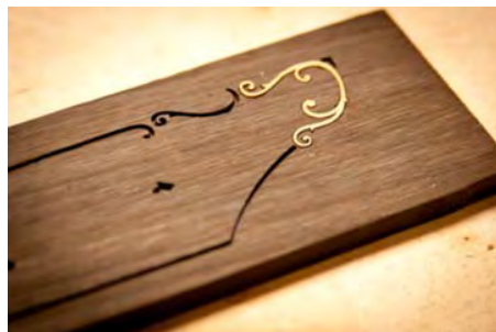
Figure 20. Incomplete Inlay (Source: www.devineguitars.com )
