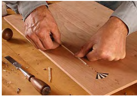
Figure 21. Inserting a long wooden piece in the vacated part of the table's surface
