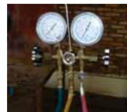
Gambar 3. Manifold Gauge
