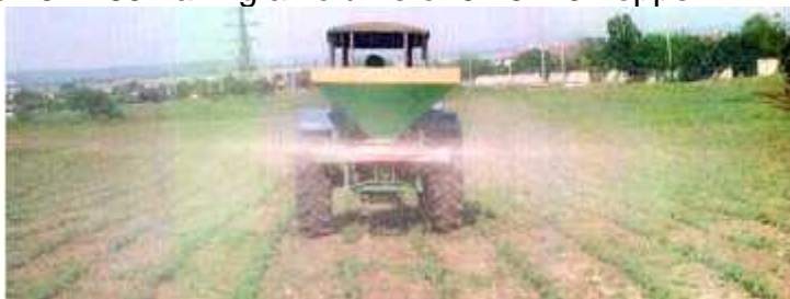
Fig. 17 - Aggregate consists of U445 tractor and car MIC 0.4M equipped with 600 mm diameter disc in work
