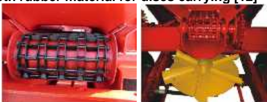
Fig. 3 - Method of regulating the flow by adjusting the rate of flow of material by means of a profiled strip [13]
