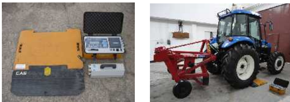
Fig. 3 – Determining weight of tractor aggregate with technical equipment for harvesting Miscanthus rhizomes [4]
