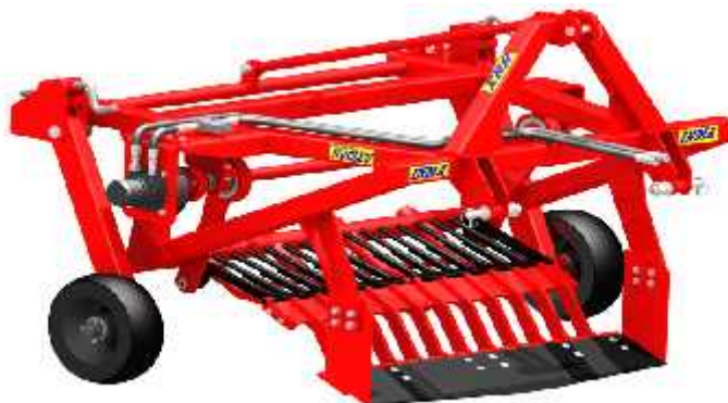
Fig. 2 - Technical equipment for harvesting Miscanthus rhizomes ERR [4]
