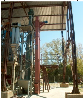
Fig.1 - Elevator with conveyor belt and buckets
