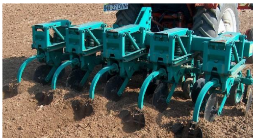
Fig. 6. Ridge cultivator equipped with shanks [28]
