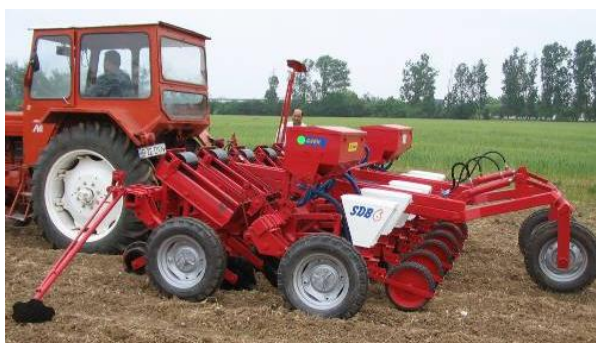
Fig. 7. Ridge sowing equipment for weeding plants [30]
