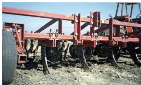
Fig. 4. Close-up view of Sundance minimum-tillage bed-conditioning implement used in the Salinas Valley [22]
