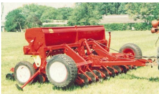
Fig. 9. Equipment for direct sowing (no-tillage) of straw cereals [5]
