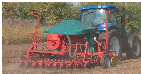
Fig. 5. Technical equipment endowed with working parts for preparing the soil and sowing straw cereals [26]
