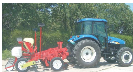
Fig. 8. Technical equipment for soil working on narrow strips, hoeing plants sowing, fertilizing and spreading insecticides [34]
