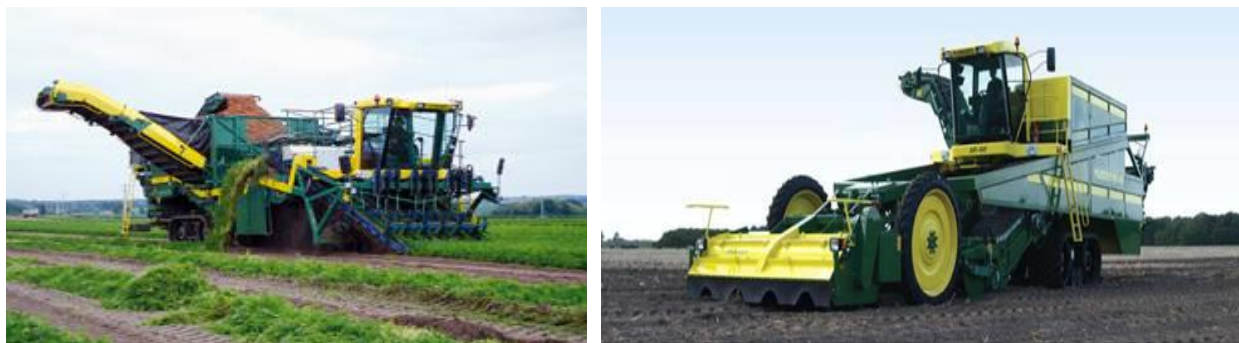
a) Ploeger carrots harvesting combine b) Ploeger potato harvesting combine Figure 11. PLOEGER carrots and potatoes harvesting combine
