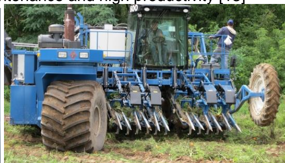
Figure 10. ASA-LIFT CM-100E combine
