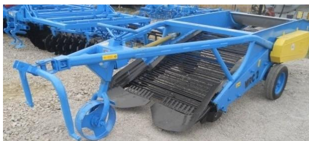
Figure 4. MRC 2 potato harvesting machine
