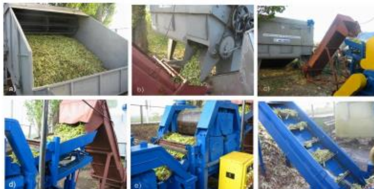
Fig.9 - Technological line for squeezing sugar sorghum [1]
