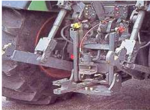
Three-point suspension mechanism Fig. 7. Rear upper coupling automatic, coupling bar [12]
