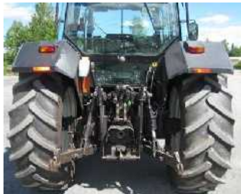
Fig. 9. Three-point suspension mechanism, rear lower coupling with hook, coupling bar [14]
