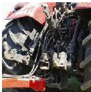
Fig. 1. Three-point linkage on a Ferguson 35 tractor / Rear three-point hitch of a Case IH tractor with implement attached by the drawbar [8]
