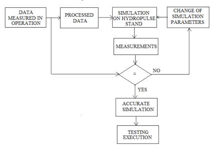
In order to achieve the physical tests is necessary to proceed sequentially through several stages:
