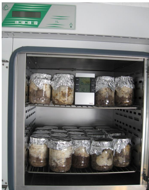
Figure 1. Glass vessels (jars) containing the lignocellulosic substrates inoculated with pure mycelia of G. lucidum și P. ostreatus , and incubated at 23°C
