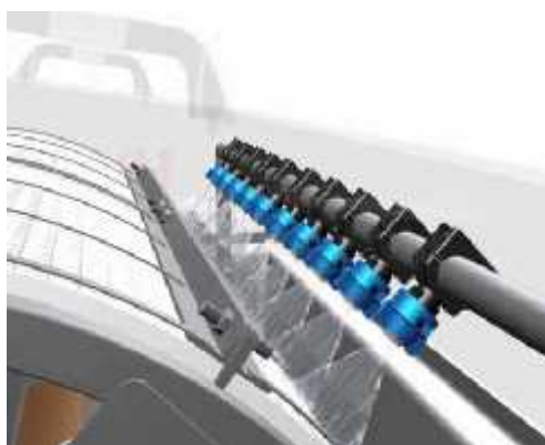
Fig. 9. Spraying systems for drum filters [27]
