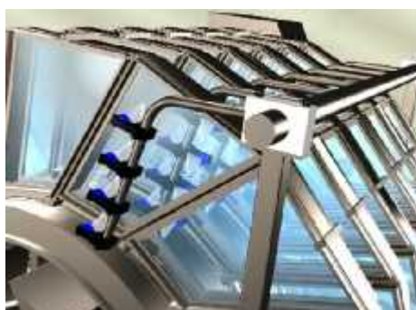
Fig.6. Spraying system for the filter with disks [26]
