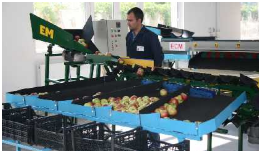
Fig.6 - Testing sorting equipment by weight–working process aspect
