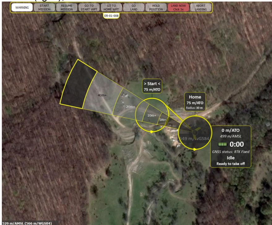
Figure 3 – Selecting the take-off and landing corridor of the drones
