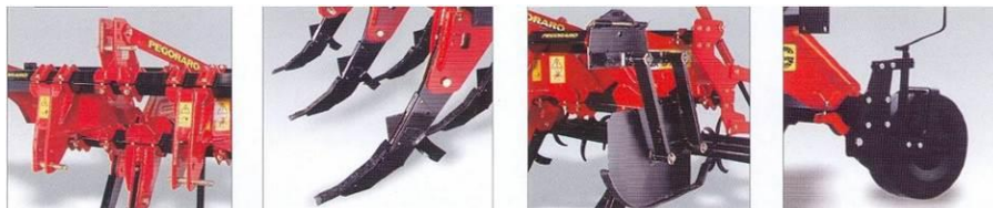
Fig. 22 - PEGORARO working bodies for deep loosening [9]
