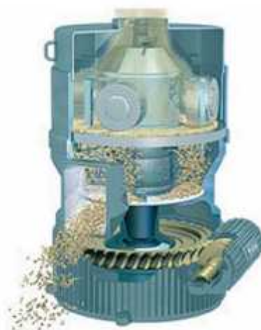
Fig. 4 – Operating principle of flat die pelletizing machines [5]
