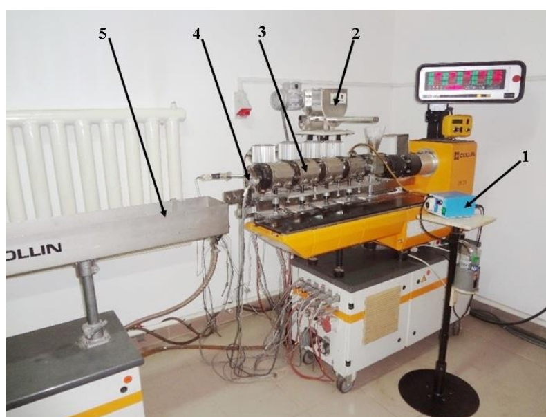
Fig.1. The installation for realization of granular fertilizer biocomposite material based on peat
