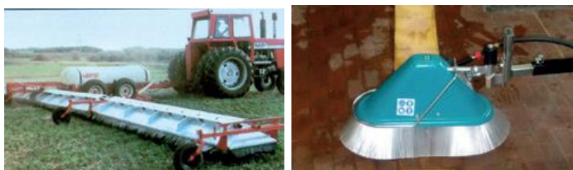
a b Fig. 8 - Shielded spraying equipment [1]
