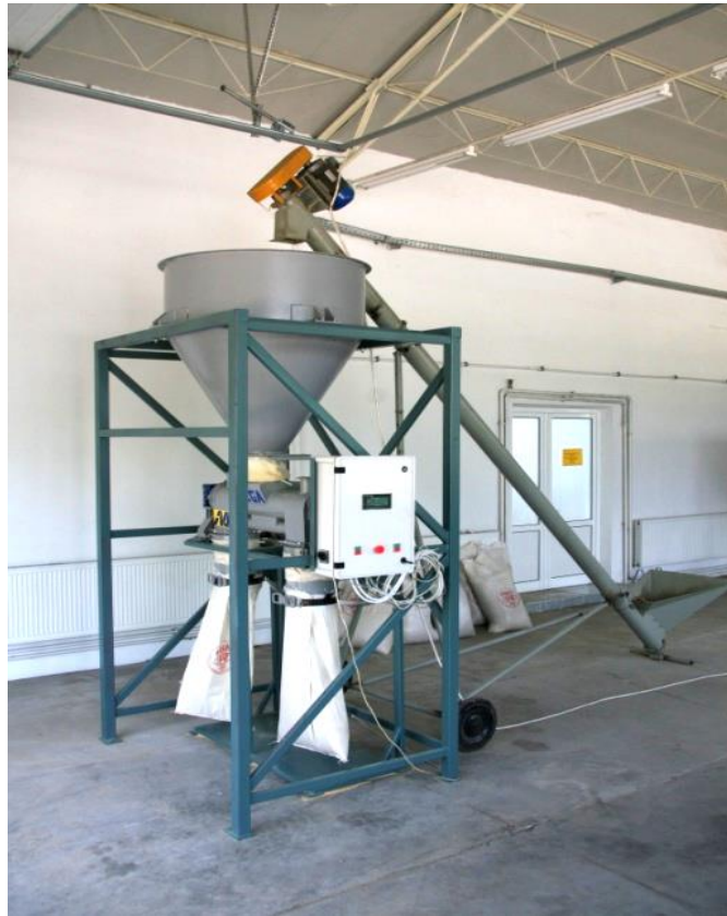
Fig. 1. – Equipment for weighing and automated management– EWAM - Overview – [2]
