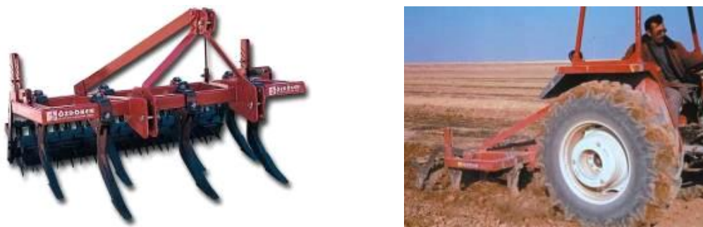
Fig. 14 – Application of vertical tillage technology with CMP chisel [8]
