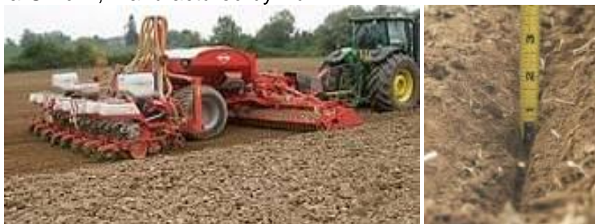
Fig. 15 – Minimum soil tillage performed with Maxima GT seeder [9]
