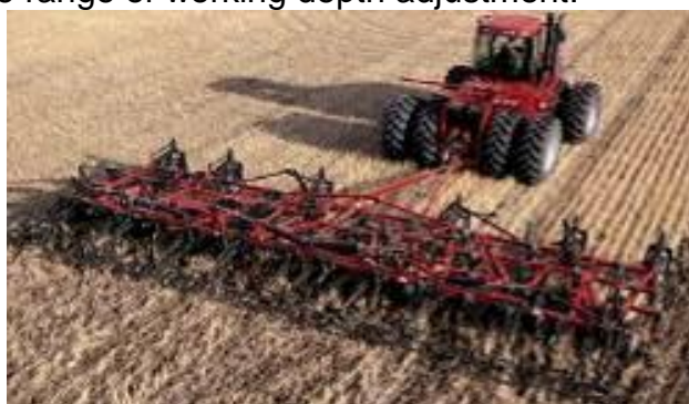
Fig. 13 – Aspects during the application of vertical tillage technology with Case IH Flex Chisel [7]
