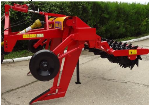
Fig. 6 – Experimental model of technical equipment with driven active bodies for deep soil loosening [4]
