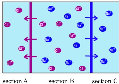
Fig. 2 Separations of ions through ion exchange membranes
