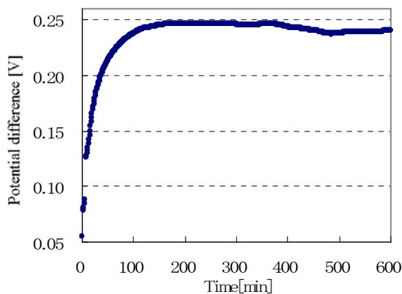
Fig. 4 Potential difference as a function of time
