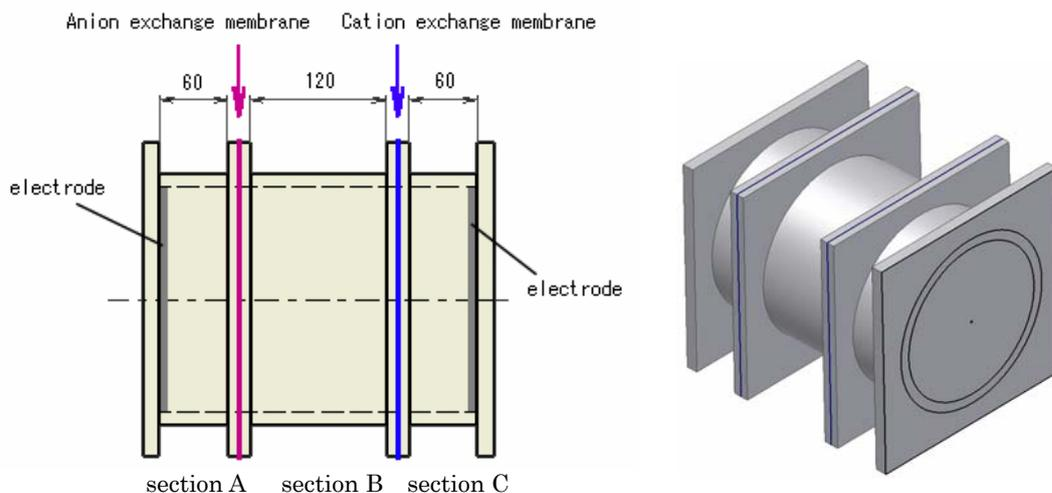
Fig. 3 The cylindrical container separating solute ions
