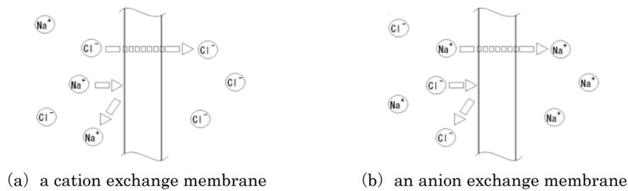
Fig. 1 Permeation through the exchange membranes
