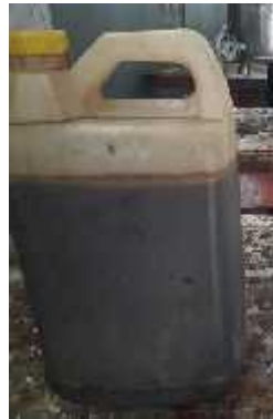
Figure 1. Polypropylene Fuel from Pyrolysis
