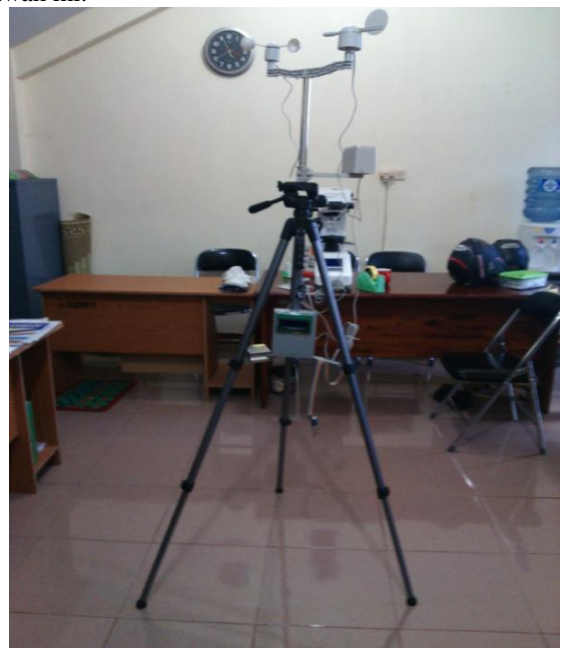
Gambar 1. Mobile Weather Station
