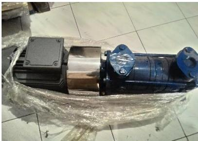
Gambar 1. Pompa Vakum VH
