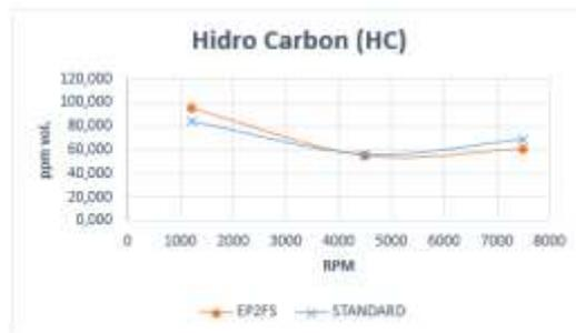
Gambar 6 Grafik volume gas buang Hidrocarbon vs rpm
