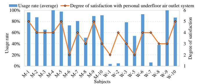
Fig. 13. Individual usage rate and satisfaction with the personal underfloor air outlet system in fall.
