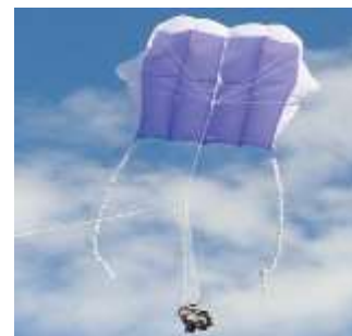
Figure 2. Unframed (parafoil) kite used for lifting the rig and camera payload (Smith et al., 2009).
