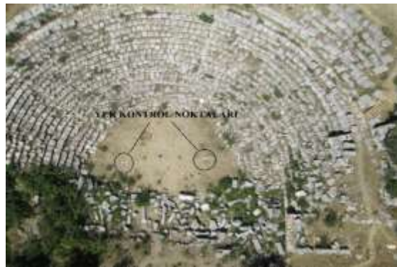
Figure 10. General view of GCP from air
