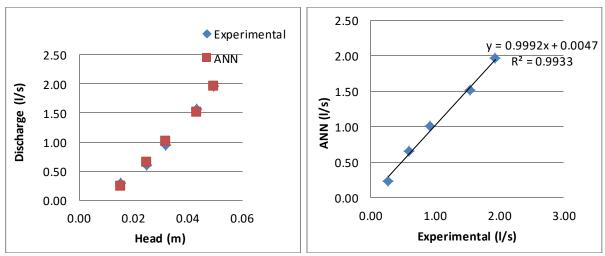
Figure 8. Relationship between the results of experimental and ANN test
