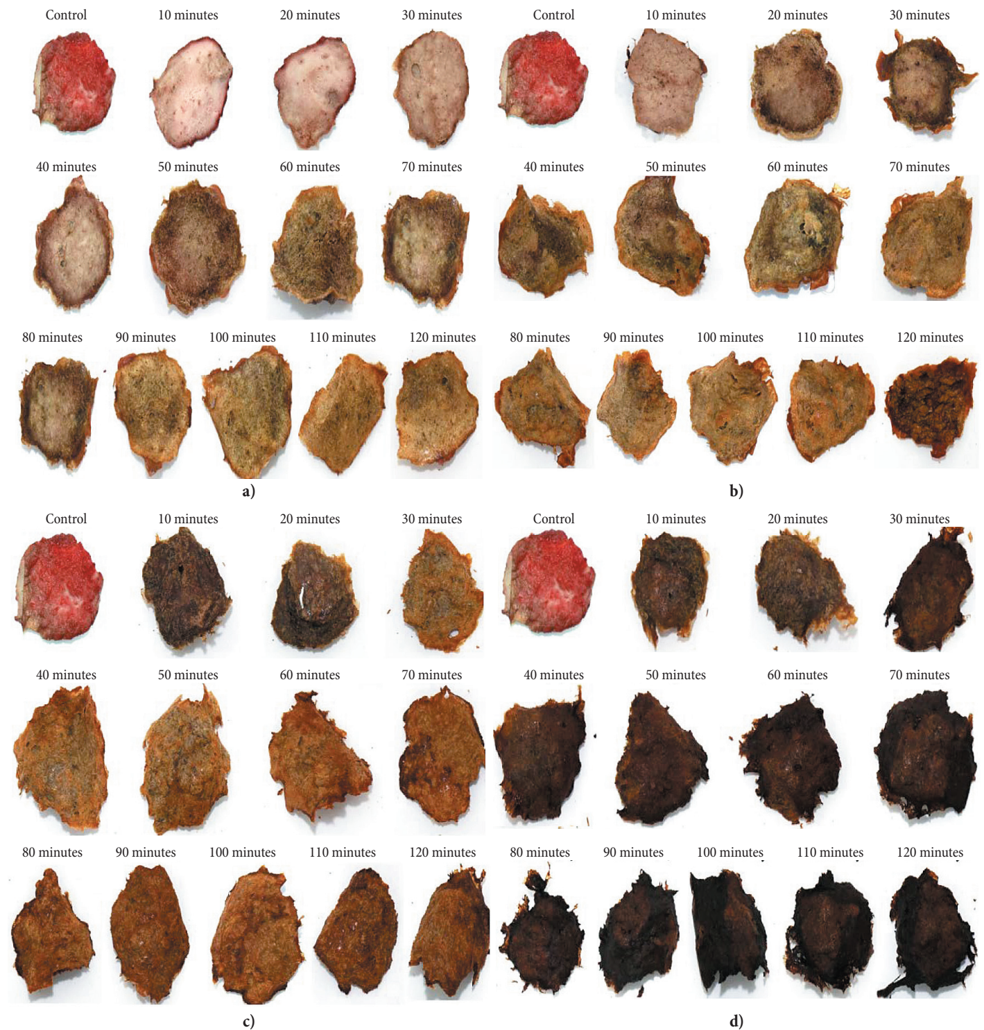
Figure 1. Beef samples subjected to heat treatment at a temperature of: a) — 120°C, b) — 150°C, c) — 180°C, d) — 210°C
