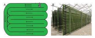
FIGURE 1. Surface view of a raceway ponds (A) and partial view of tubular photobioreactor (B) used for microalgae cultivation (Modified from Abomohra *et al.*, 2016).
