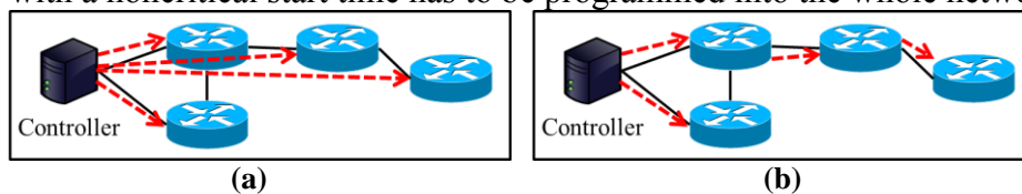
Figure 3. (a) Regular flow installation: from controller to each network equipment. (b) The flow installation using the proposed network equipment to equipment flow installation.
