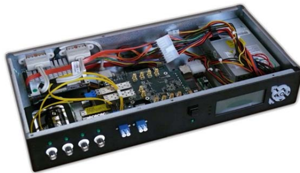
Figure 1: Working sample of a two-way transfer adapter
