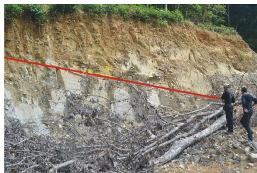
Figure 3: Outcrop of slate with characteristic yellowish gray color with a thick laminated. Shows strike 330^\circ\text{E} and dip 14^\circ .
