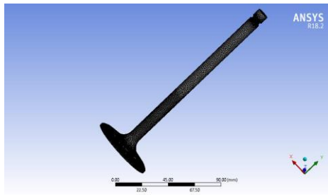
Fig.10 Mesh of valve with sodium and TiCN coating
