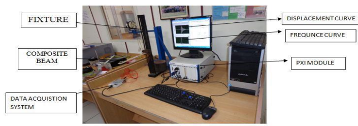
Fig. 7: Representation of Forced Vibration Testing apparatus
