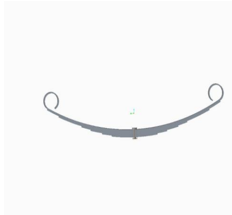
Fig 2. leaf spring designed in CATIA
