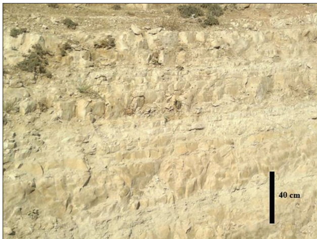
Figure 5. Part of the exposed rocks in the sampled section of the Pila Spi Formation. Note the nature of the bedding and their thicknesses.
