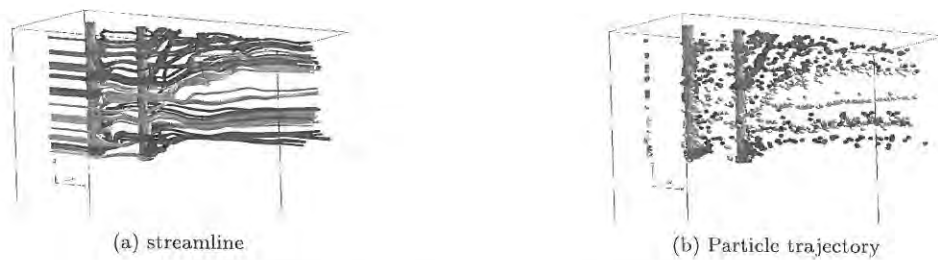
Fig 6 Upward flow motion observed behind two circular cylinders
