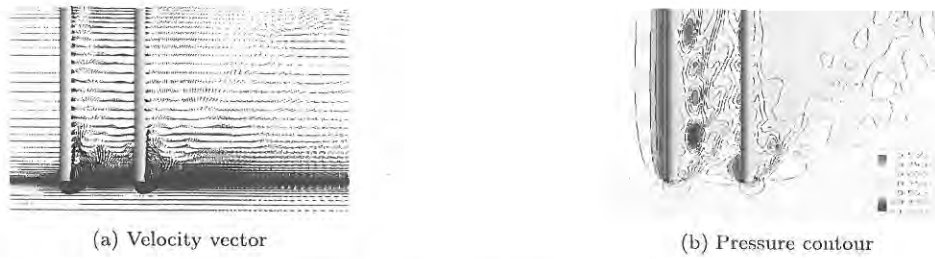
Fig 4 Computed results on x-z plane across circular cylinders
