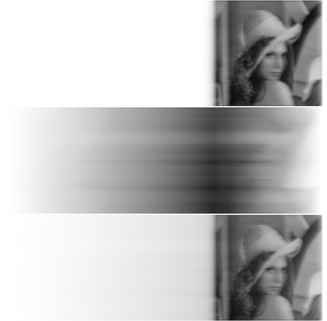
Fig. 4: Effects of the fractional integral on a moving object (from left to right): Top: effects of a fast feedback loop. Middle: effect of a slow feedback loop. Bottom: Weighted sum of the top and middle images: approximation of fractional integral I^{0.2} , the same as the VPs activity.
