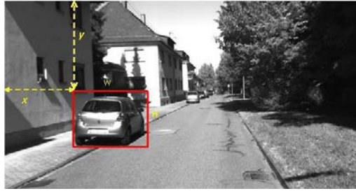
Figure 5: Figure shows the parameters used in the Kalman filter. They are the coordinates of the object's top left point (x, y) and the size (width (w) and height (h) ) of the object.
