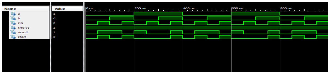
Figure 5(b): Waveforms of Proposed work (Full Subtractor)
