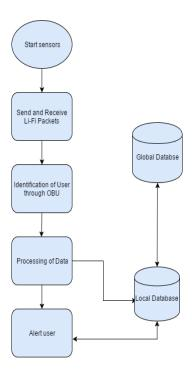
Figure 4: System Flowchart for Infrastructure-less Vehicular Communication System
