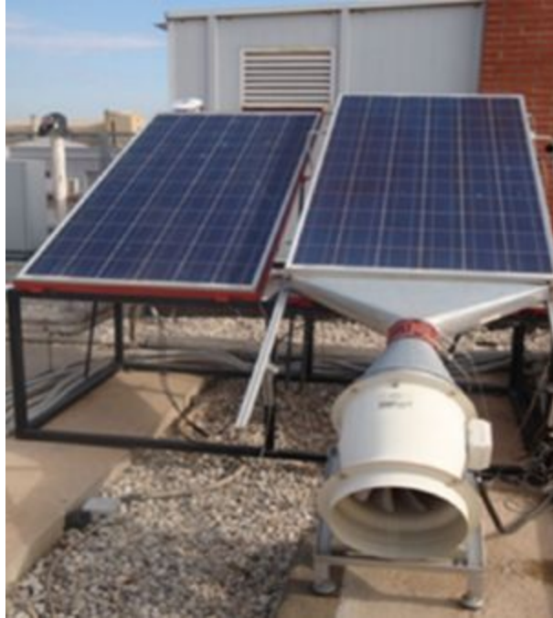
Figure 2. Forced air cooling [7]
