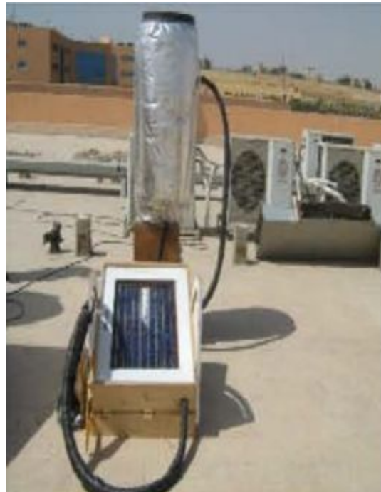
Figure 4. PV/T with Thermosyphon[11]
