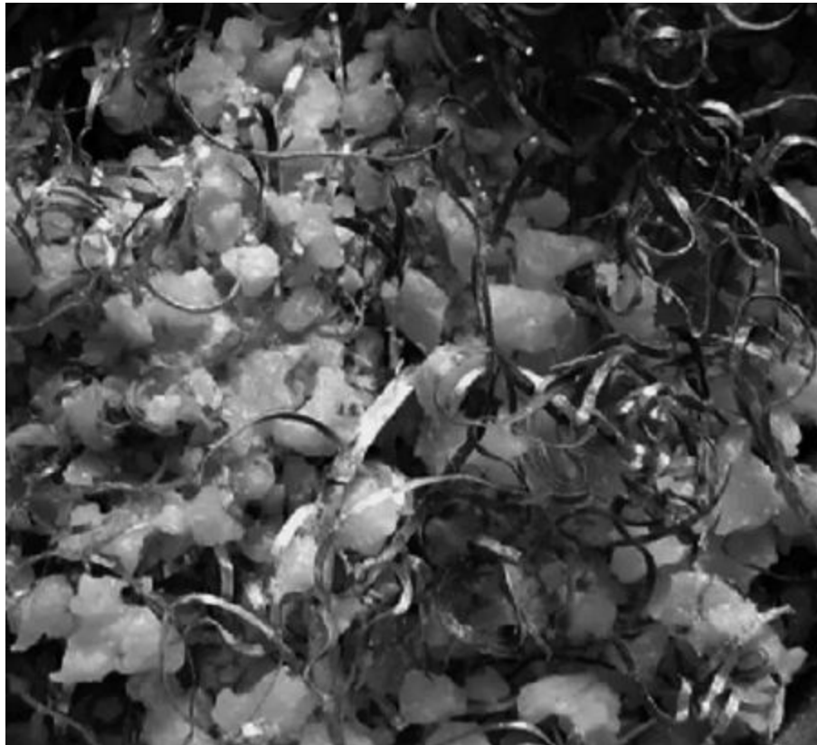
Figure 5. PCM and Aluminum shaving used for PV cooling [13]
