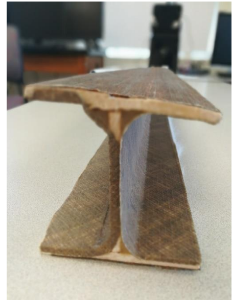
Figure 20: Beam with crushed webbing and flanges
