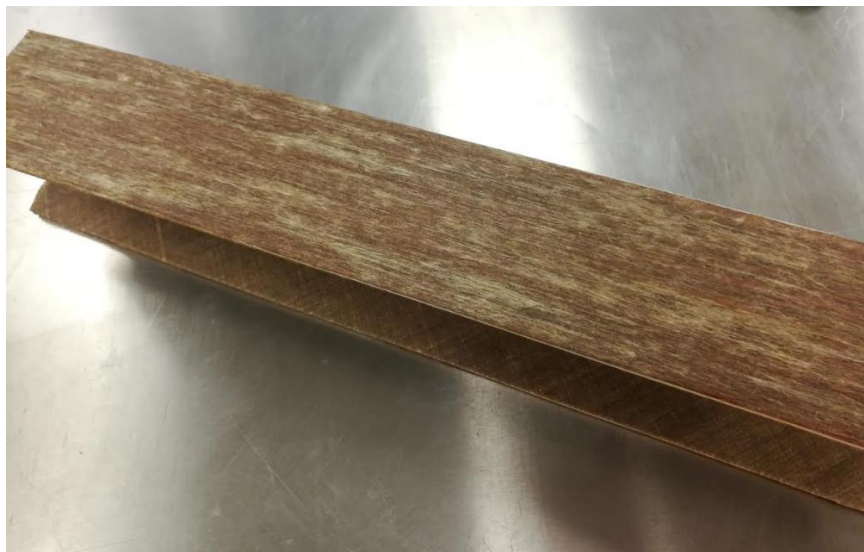
Figure 21: Beam that lost vacuum during production resulting in top fibers not wetting through the layer.
