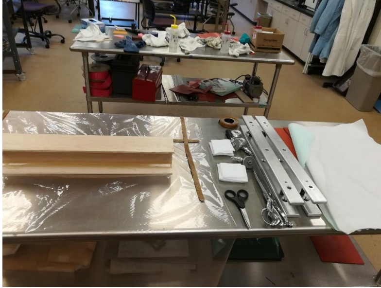
Figure 12: Beam with associated consumables waiting for fiber composite to be applied.
