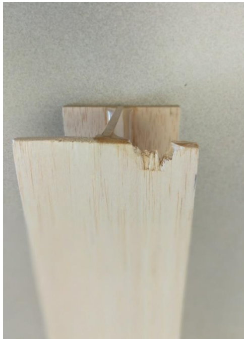
Figure 18: Beam produced with broken balsa.
