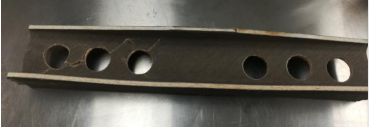
Figure 23: Picture of beam produced for competition. Failure at left Holes.
