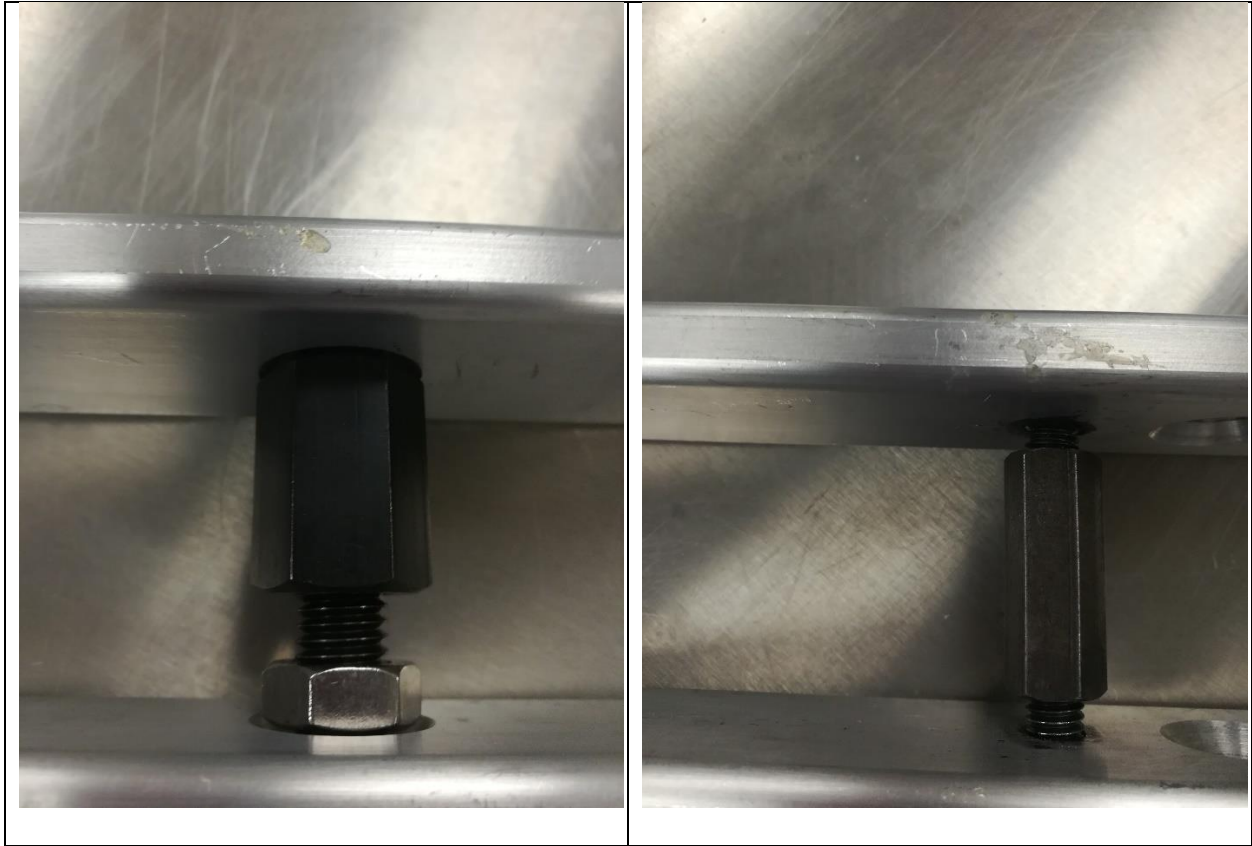
Figure 13: Old method to adjust flange tooling (left) and new method (right)
