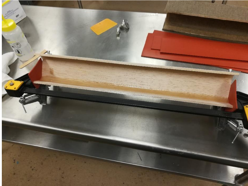
Figure 11: Making epoxy fillet at inner corner of I-beam
