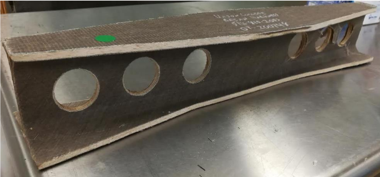
Figure 22: Picture of beam produced for competition. Failure at right hand holes.
