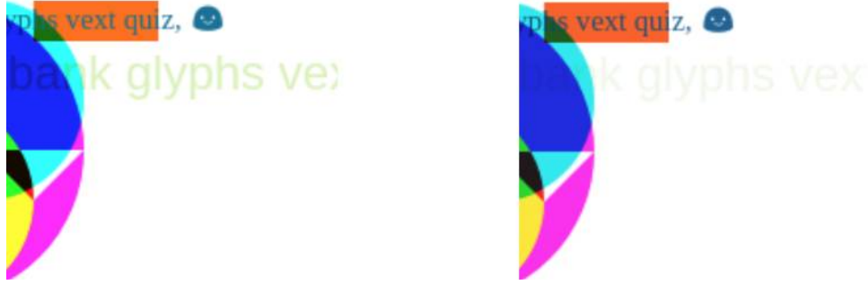
Figure 4: On the left side of the image above is a portion of a canvas fingerprint rendered from an unmodified browser. On the right side is a portion of a canvas fingerprint rendered from a browser with just our color randomizations implemented. This highlights the visible difference in output caused by our randomizations in the R, G, B and A properties.
