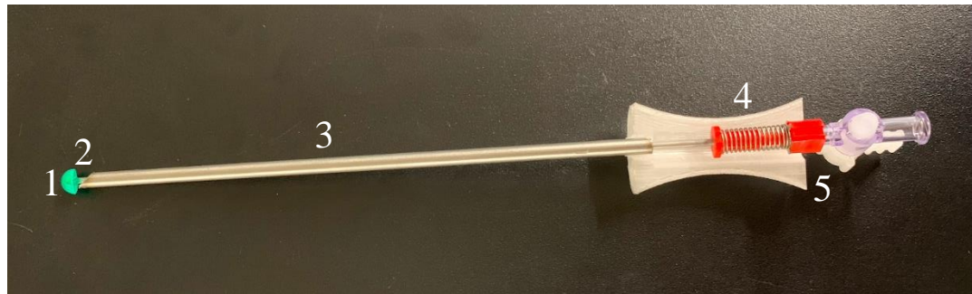
Figure 6. Final prototype iteration. The buffer (1), stylet (2), cannula (3), spring (4), and handle (5) fit together to create a working prototype. The handle is shown in a cross sectional view.
