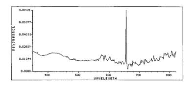
Figure 3-2: Absorption spectrum of MB post-doped Slide-9MeOH after soaking in  $SO_3^{-2}$  solution.
