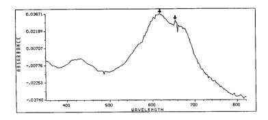
Figure 3-1: Absorption spectrum of MB post-doped Slide-9MeOH.
