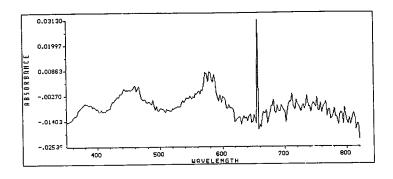
Figure 3-3: Absorption spectrum of MB post-doped Slide-9MeOH after soaking in  $H_2O_2$  solution.
