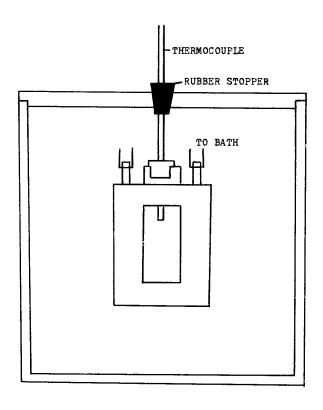
an Omega 2160A digital thermometer directly in the sample cell. To allow this, it was necessary to drill a hole in the cell compartment cover of the Cary 118C. The thermocouple was inserted through a rubber stopper which in turn was inserted securely in the hole in the cell compartment cover. The tapered rubber stopper did not allow any light leaks into the cell compartment. The teflon cap of the sample cell was also drilled to allow passage of the thermocouple into the sample solution.
