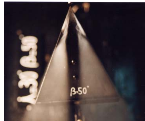
Photograph 3b : Visualisation of air flow on the upper surface of the Delta baffle bent longitudinally at an incidence i of 60^\circ , viewed from above
